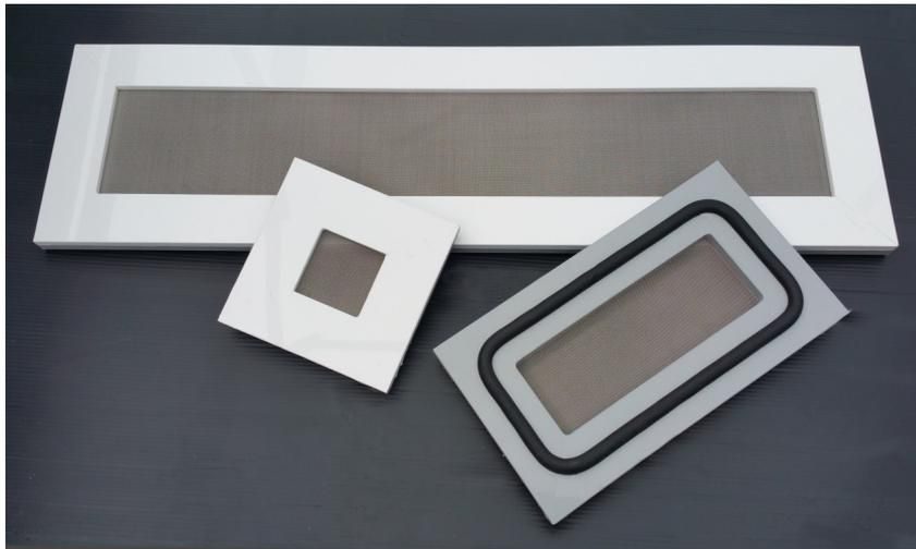
Testing conducted under the auspices of “Advanced Filtration” on 2nd September, 2016 at their premises on their test equipment to determine the pressure drop generated by the two meshes when placed in a duct and subjected to varying air velocities, provided the following data as tabulated below:
