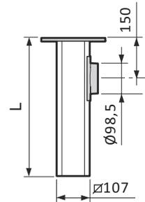
Ceiling bracket, for fitting through beams. The attachment plate is adjustable for the entire length of the aluminium profile. If required, the aluminium profile can be cut during fitting.
