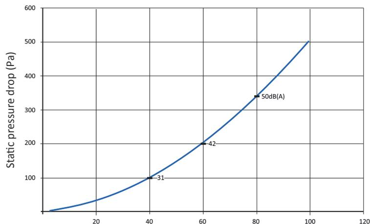
Static pressure drop is measured in accordance with ISO standard 5167-1. Air flow (m<sup>3</sup>/h)
